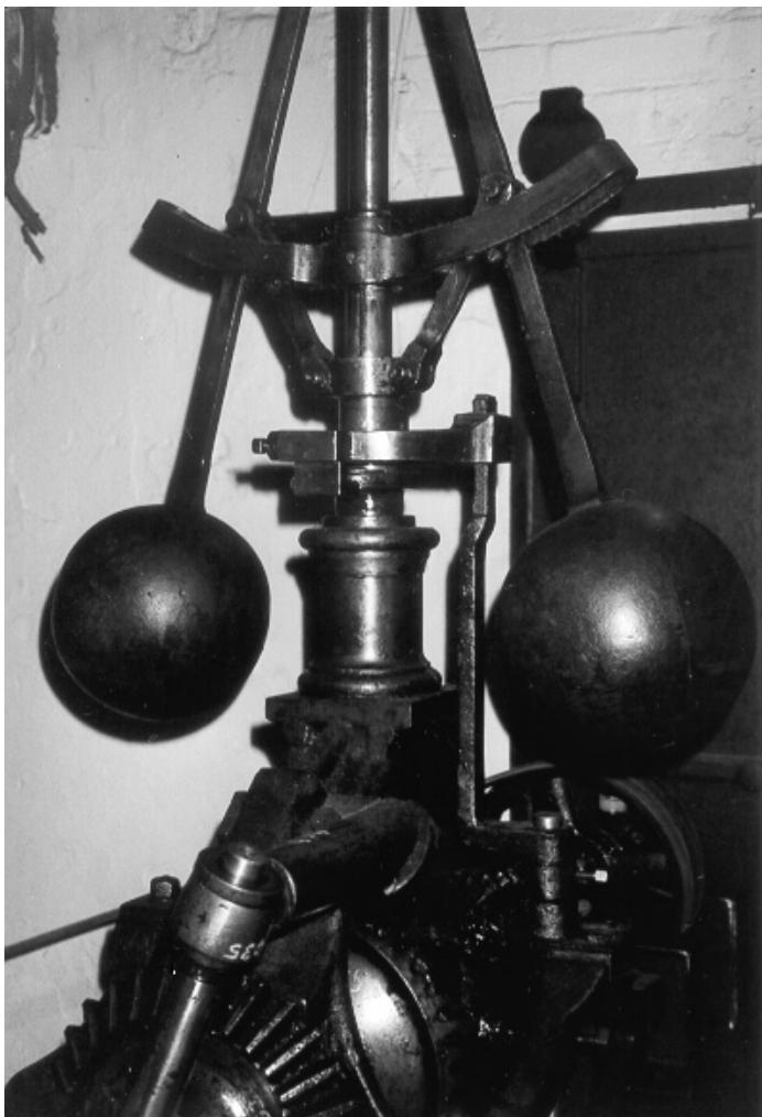
This flyball governor is in the same cotton factory in Manchester. However, this particular governor was used to regulate the speed of a water wheel driven by the flow of the river. The governor is quite large as can be gauged by the outline of the door frame behind the governor.
