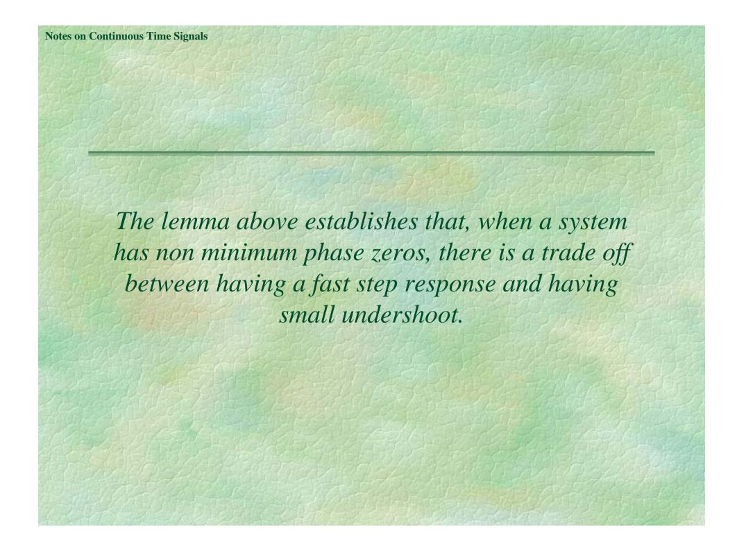
Slow zeros and overshoot. Assume a linear, stable system with transfer function H(s) having unity d.c. gain and a zero at s=c, c<0. Define v(t)=1-y(t), where y(t) is the unit step response. Further assume that
