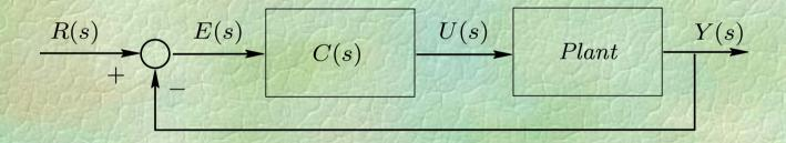
Figure 6.1: Basic feedback control loop
