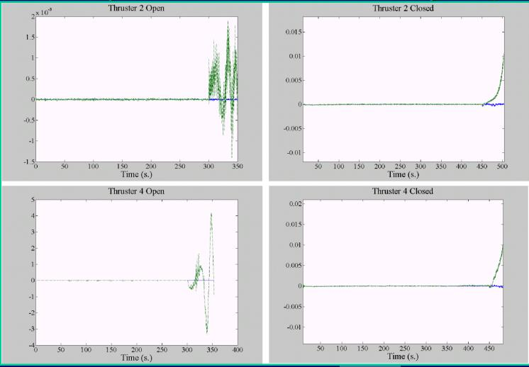
Fault-free & faulty residuals for thruster faults.
