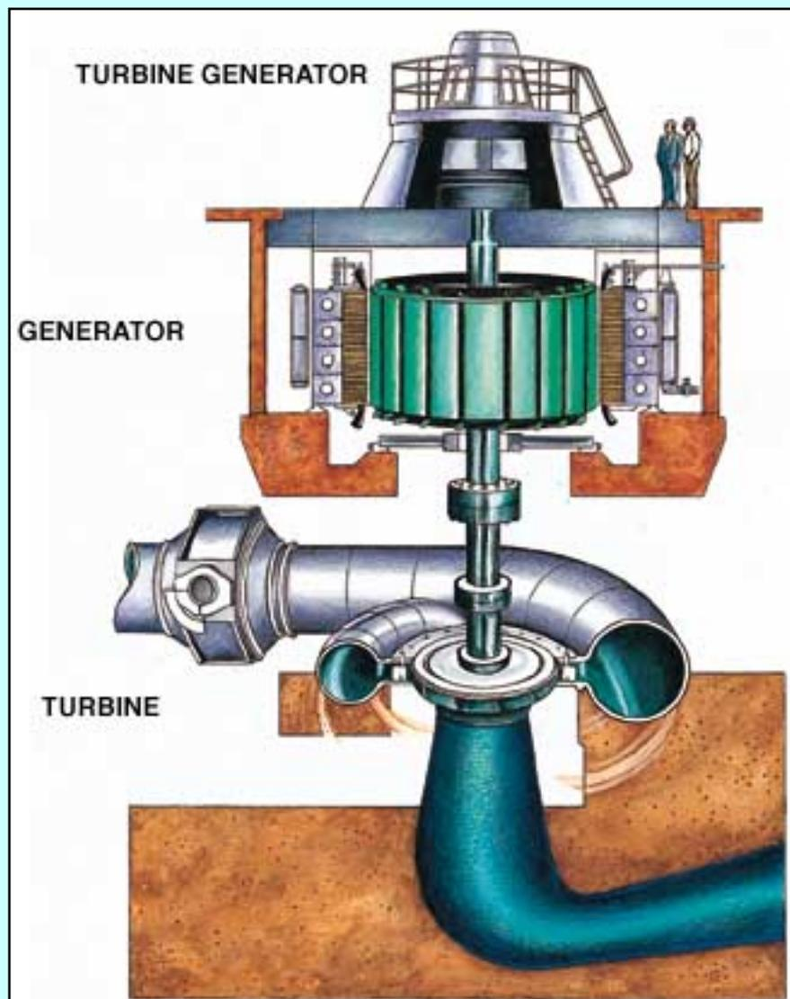
Flowing water is directed at a turbine (remember turbines are just advanced waterwheels). The flowing water causes the turbine to rotate, converting the water's kinetic energy into mechanical energy.
