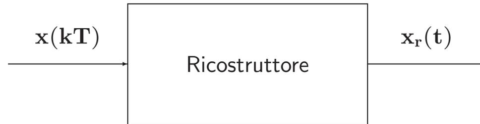
$$x_r(t) = x(kT) + \left. \frac{dx(t)}{dt} \right|_{t=kT} (t - kT) + \left. \frac{d^2 x(t)}{dt^2} \right|_{t=kT} \frac{(t - kT)^2}{2!} + \dots$$
