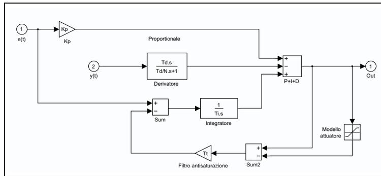
Figura 6.20: PID in *Simulink* a derivata limitata e anti-windup.
