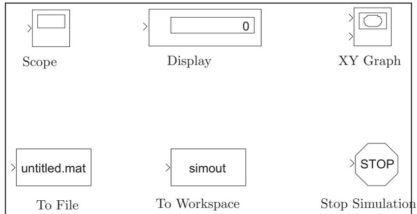
Figura 2.3: *Simulink* Signal Sinks library.
