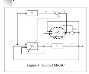
The **neural network**  $NN_M$  is trained to approximate the plant G input/output relation using the signal  $e_M$ . This is usually done offline, using a batch of data gathered from the plant in open loop.
