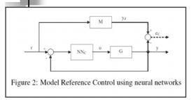
The signal  $e_C$  is used to train or adapt online the weights of the controller  $NN_C$ . Two are the approaches used to design a MRAC control for an unknown plant: **Direct and Indirect Control**.
