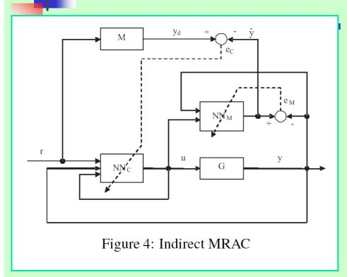
This approach uses neural two networks: one for modelling the plant dynamics  $(NN_M)$ , another and one trained to control the real plant (G) so as its behaviour is as close as possible to the reference model (M) via the neural controller  $(NN_C)$ .
