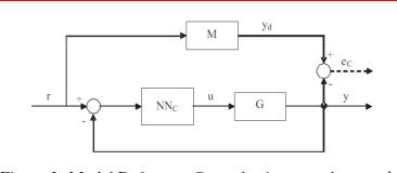
Figure 2: Model Reference Control using neural networks
