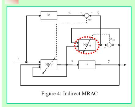
The neural network  $NN_M$  is trained to approximate the plant G input/output relation using the signal  $e_M$ . This is usually done offline, using a batch of data gathered from the plant in open loop.
